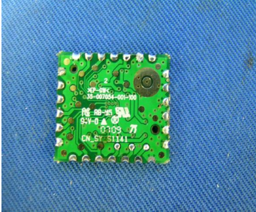
Base Unit Bluetooth RF Module rear side
