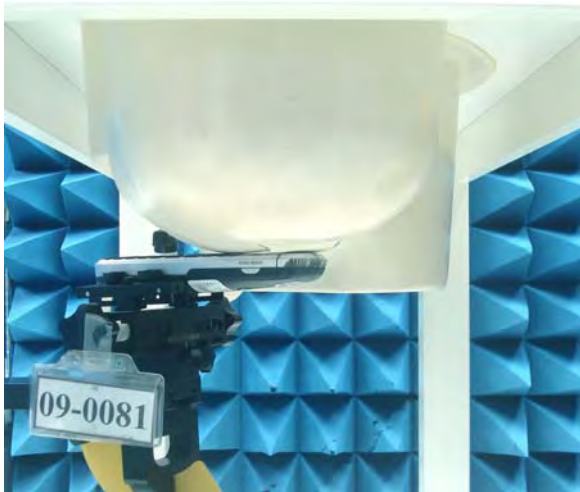
Figure 16. Left Head SAR Test Setup (Cheek)
