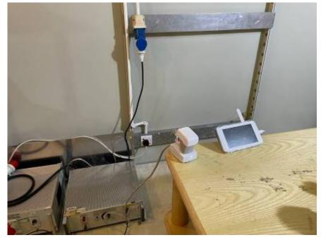
Radiated Emissions (30MHz-1GHz) Test Setup
