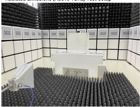
Radiated Emissions (Above 1GHz) Test Setup
