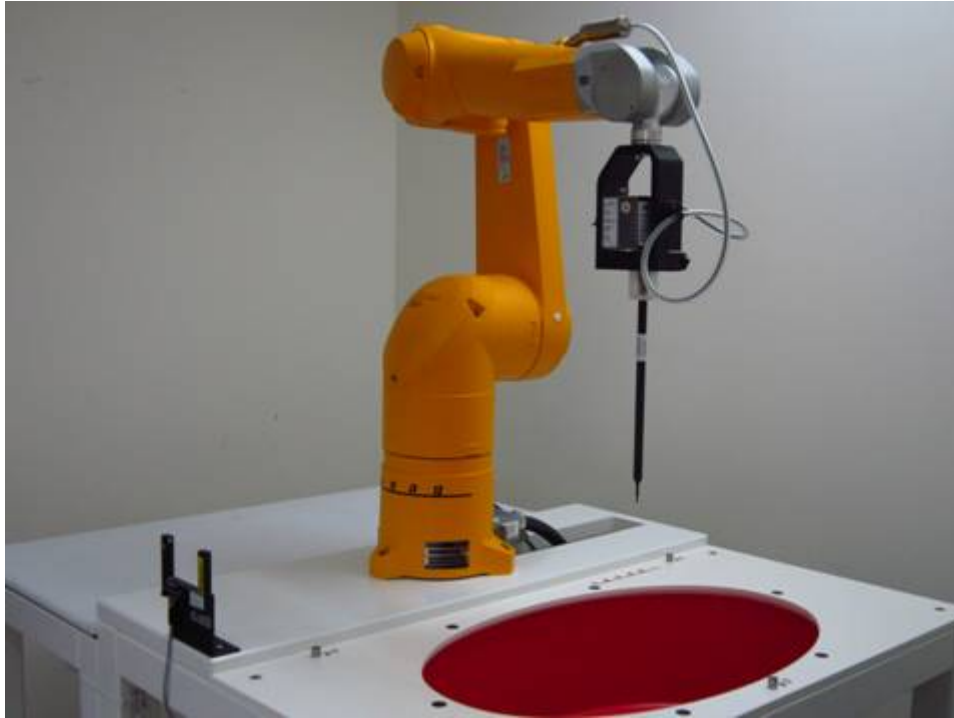
Fig.1 Photograph of the SAR measurement system
