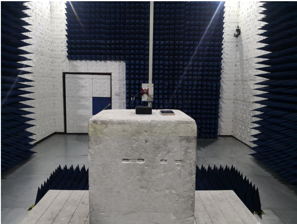
RADIATED EMISSION TEST SETUP ABOVE 1GHZ
