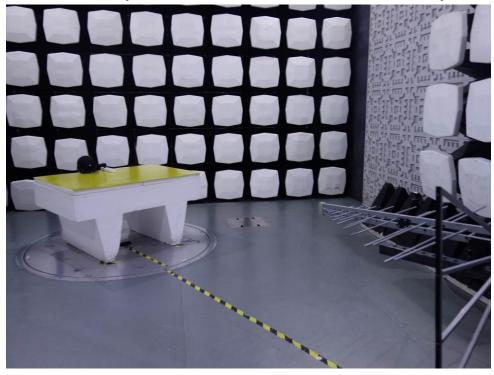
1.3 Radiated Spurious Emissions above 1GHz Test Setup
