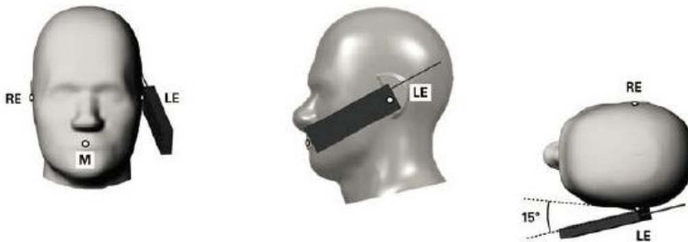
Fig.11.4 Illustration for Tilted Position
