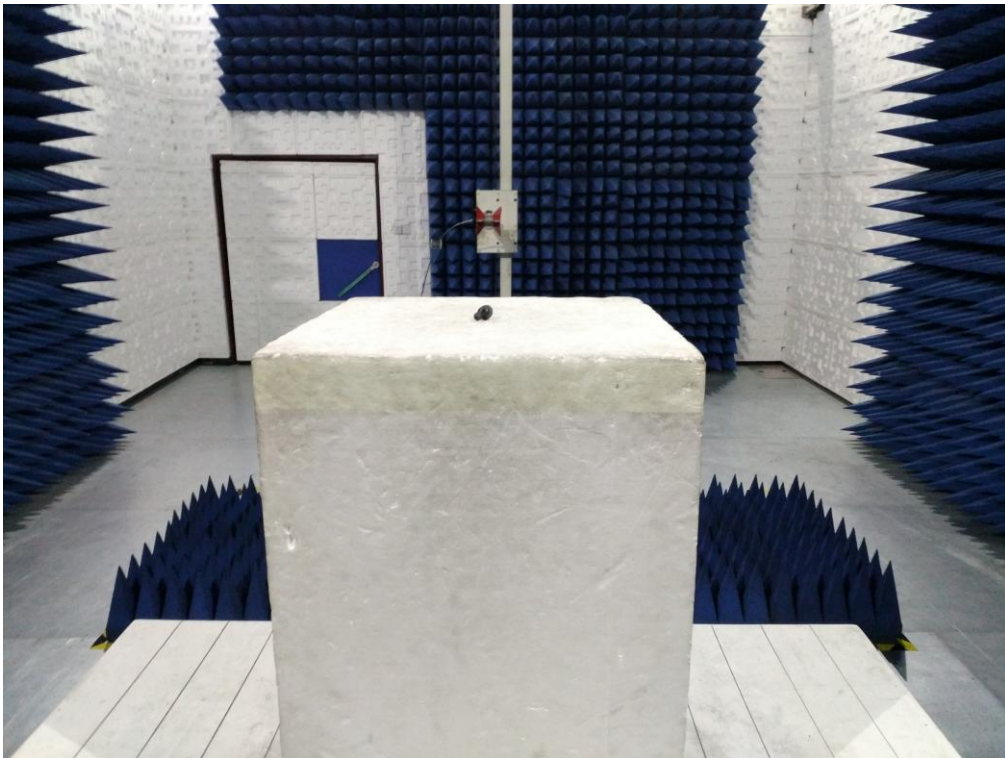
RADIATED EMISSION TEST SETUP ABOVE 1GHZ
