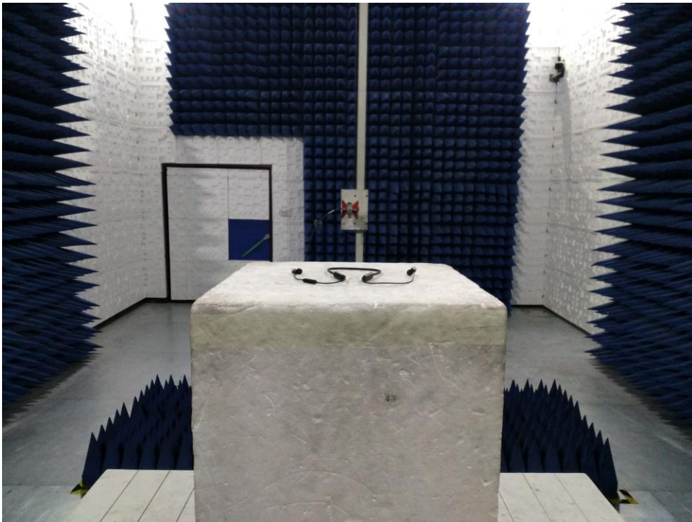
RADIATED EMISSION TEST SETUP ABOVE 1GHZ
