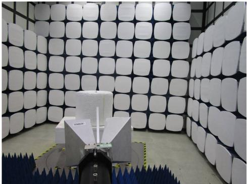
1.2 Radiated Spurious Emissions Test Setup
