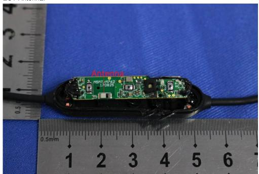
The antenna is integrated on the main PCB and no consideration of replacement. The best case gain of the antenna is 1dBi.
