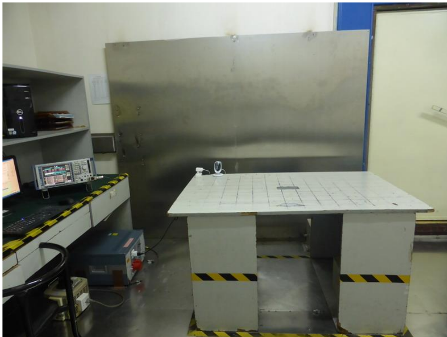
Photograph 4: Set-up for Conducted Emission on AC Mains
