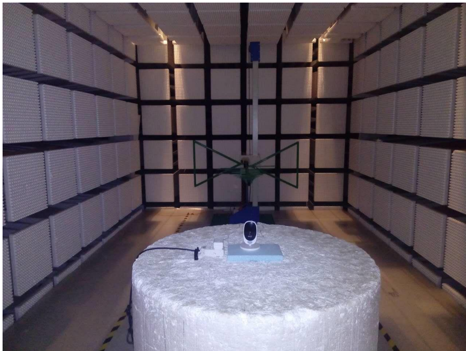
Photograph 2: Set-up for Radiated Spurious Emission, 30MHz ~ 1GHz
