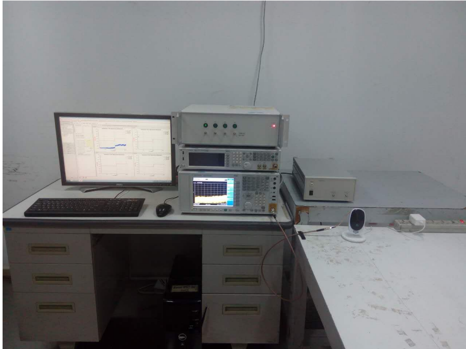
Photograph 1: Set-up for Radio Spectrum Test
