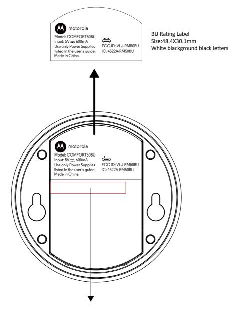
SN Label stick on the back of stand Size:40X6mm
