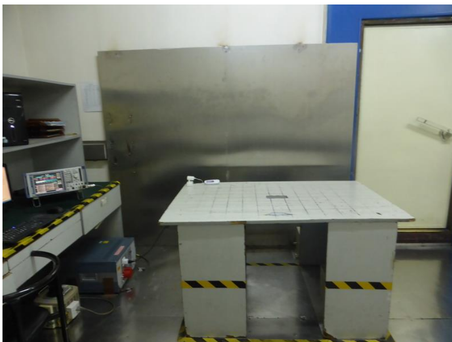
Photograph 4: Set-up for Conducted Emission on AC Mains
