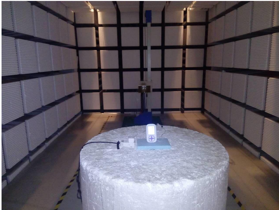
Photograph 3: Set-up for Radiated Spurious Emission, 1GHz ~ 26.5GHz
