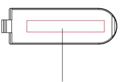
SN Label stick on the back of stand Size:40X6mm
