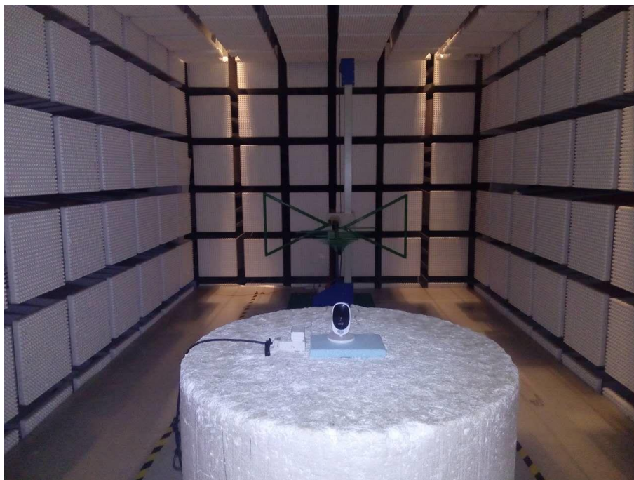
Photograph 2: Set-up for Radiated Spurious Emission, 30MHz ~ 1GHz
