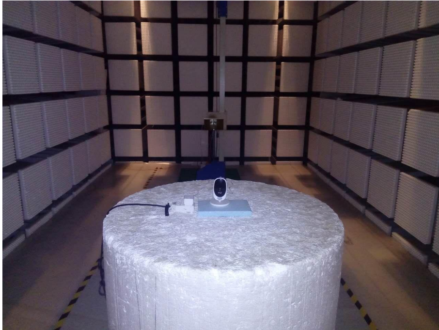
Photograph 3: Set-up for Radiated Spurious Emission, 1GHz ~ 26.5GHz
