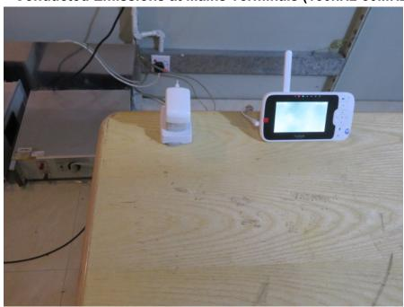
Radiated Emissions (30MHz-1GHz) Test Setup
