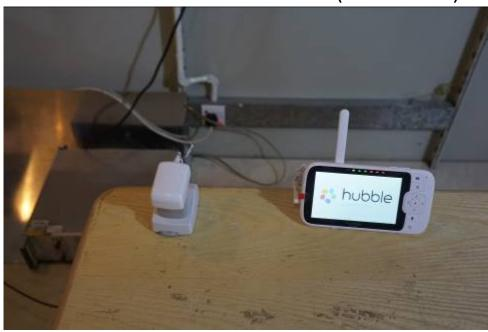
Radiated Emissions (30MHz-1GHz) Test Setup
