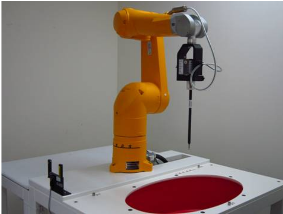
Fig.1 Photograph of the SAR measurement system
