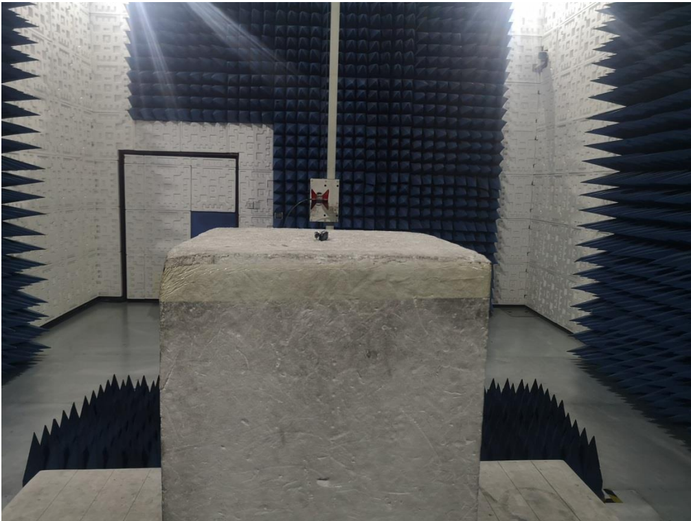
RADIATED EMISSION TEST SETUP ABOVE 1GHz
