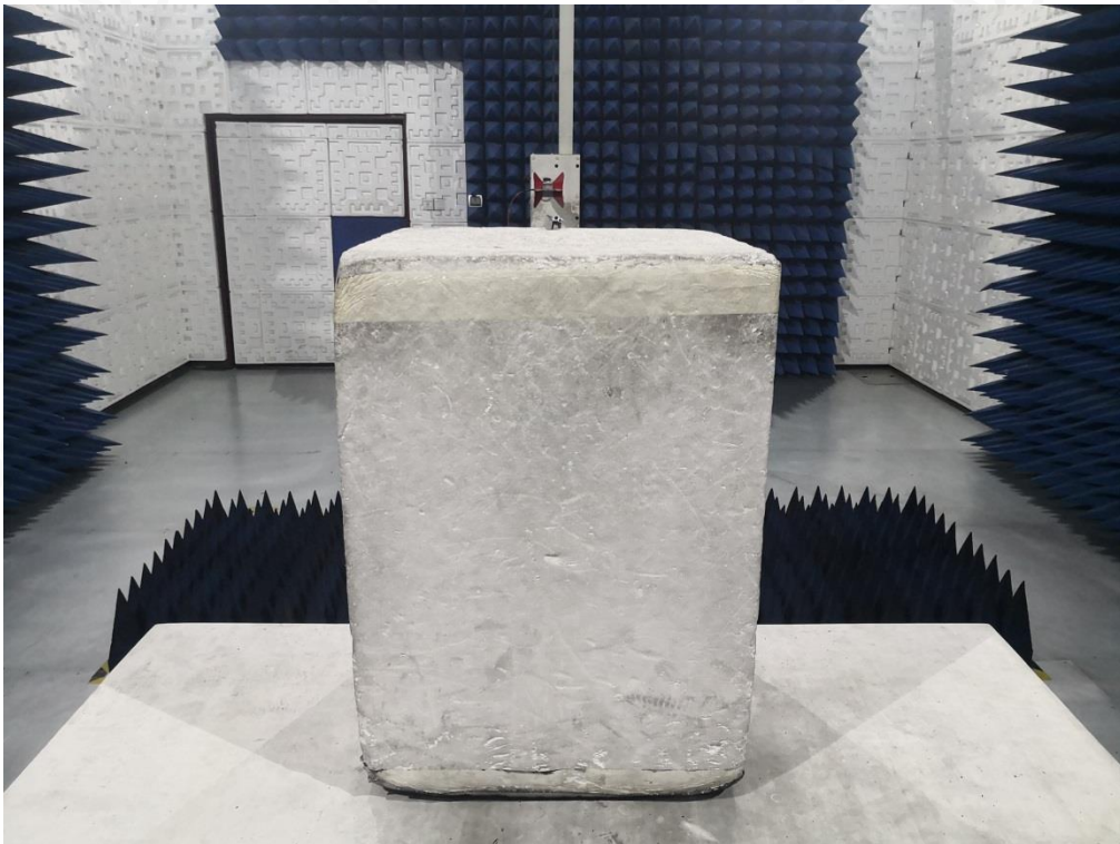
RADIATED EMISSION TEST SETUP ABOVE 1GHz
