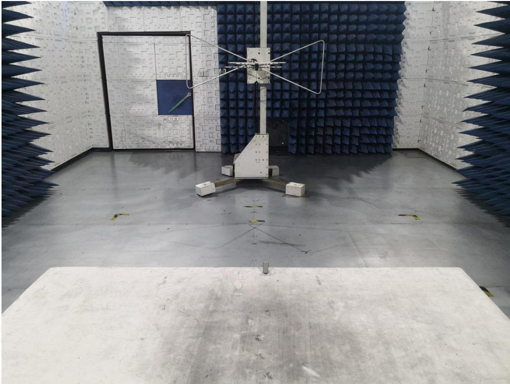
RADIATED EMISSION TEST SETUP ABOVE 1GHz
