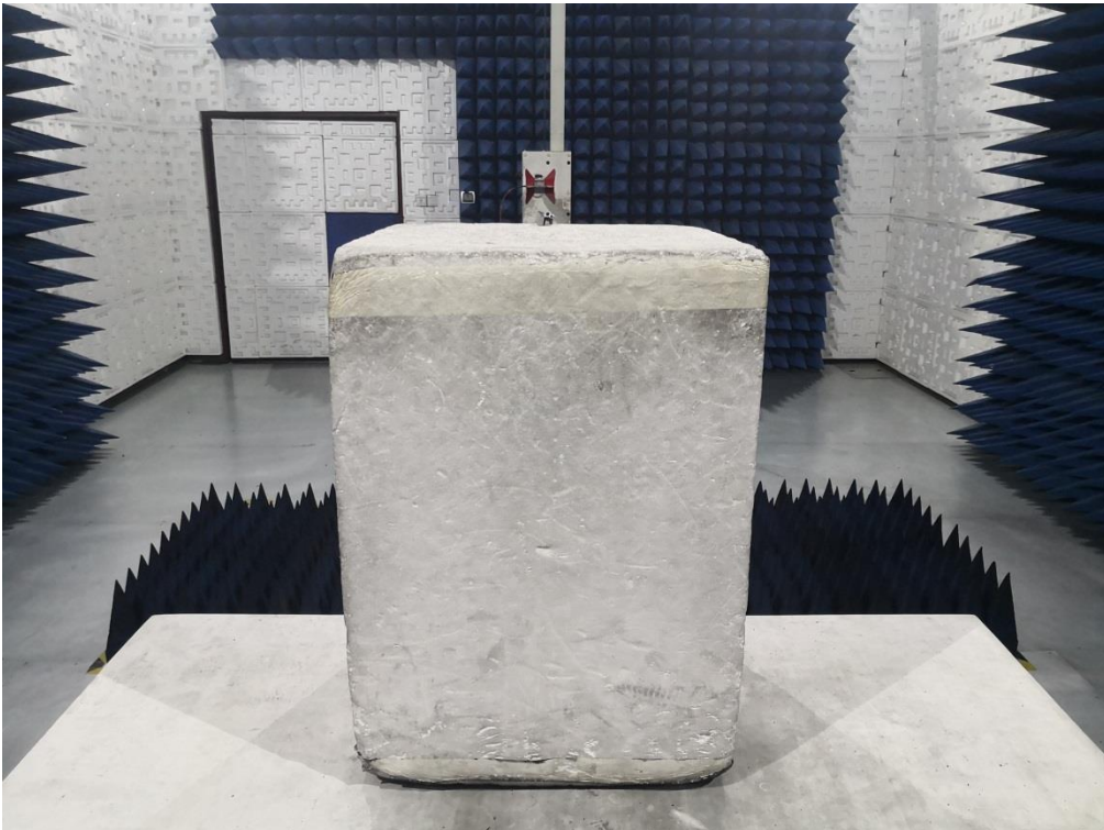
RADIATED EMISSION TEST SETUP ABOVE 1GHz
