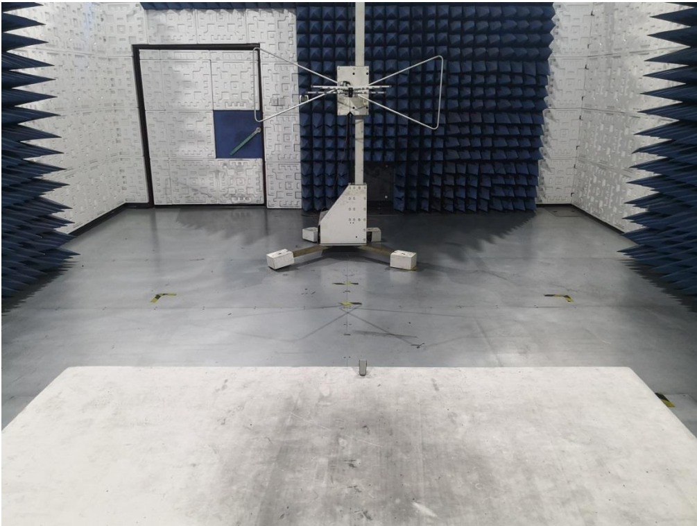
RADIATED EMISSION TEST SETUP ABOVE 1GHz
