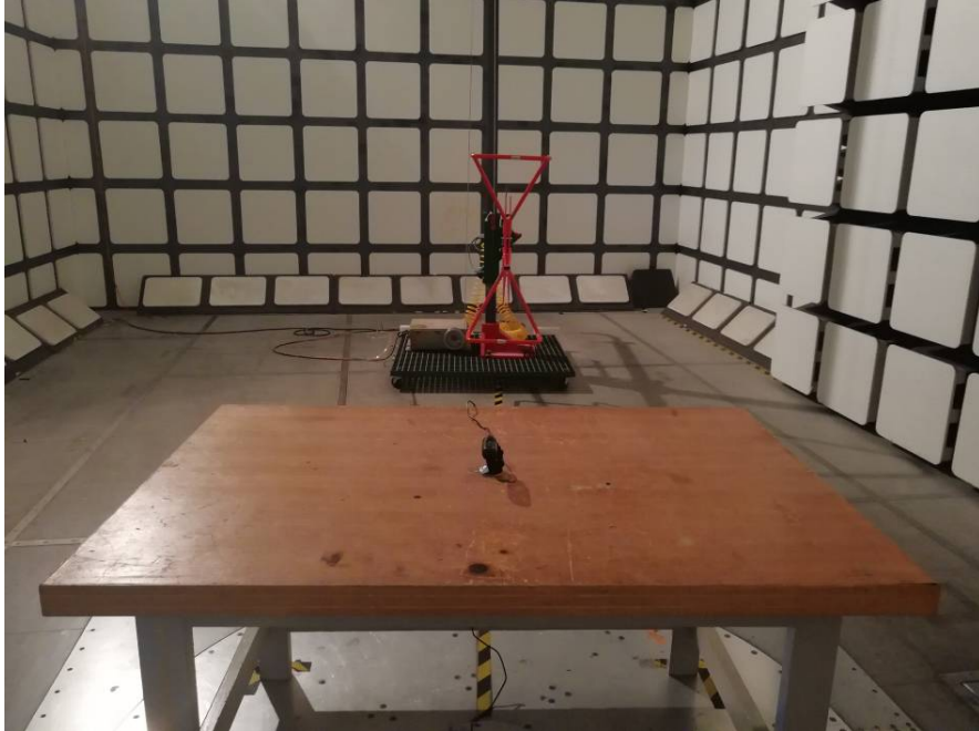
Radiated Emissions View (Below 1 GHz)
