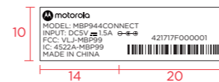
FCC/IC Label Size: 34L x 10H mm Printing: Black color Material: adhesive label with plastic lamination
