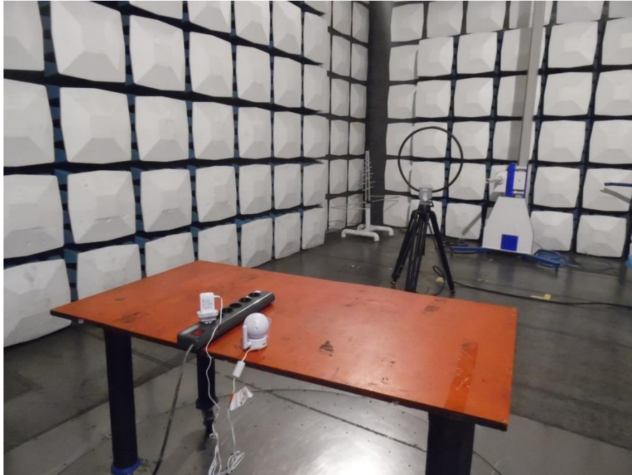
Photograph 1: Set-up for Radiated Spurious Emission, 9kHz - 30MHz
