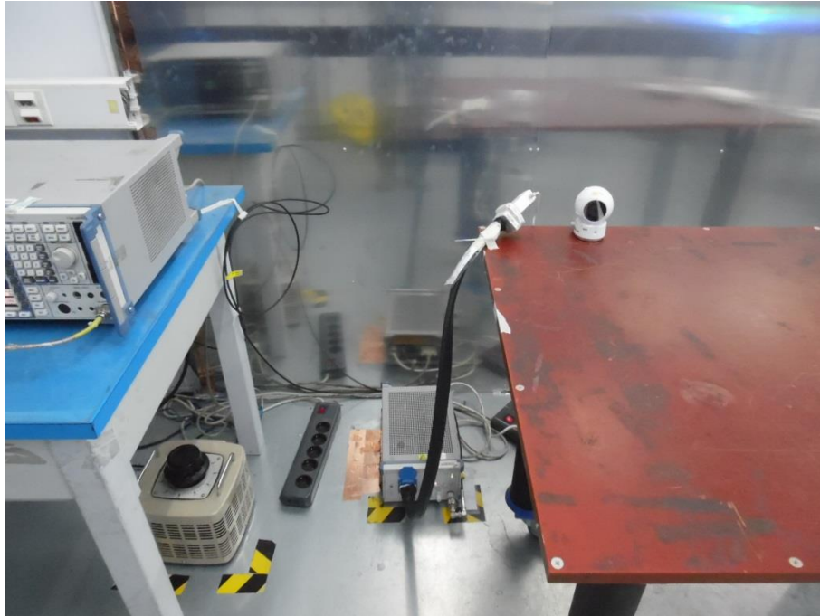
Photograph 5: Set-up for Conducted Emission on AC Mains
