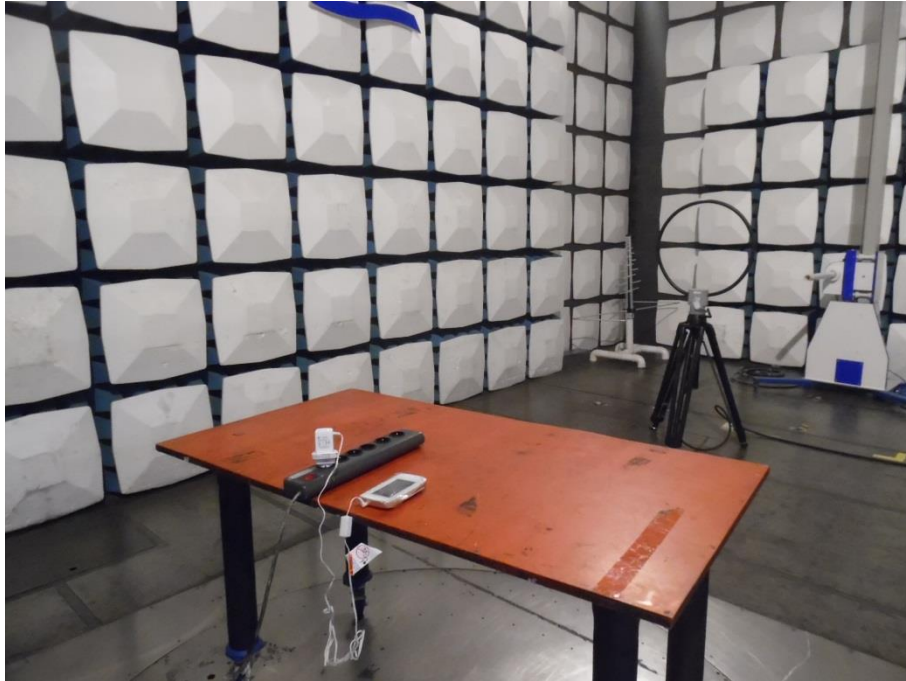
Photograph 1: Set-up for Radiated Spurious Emission, 9kHz - 30MHz
