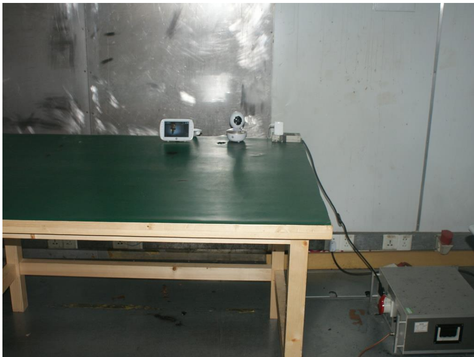
Photograph 4: Set-up for Conducted Emission on AC Mains
