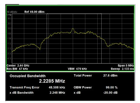
Result data graph shows 20 dB bandwidth, CF = 2440MHz, BW = 2.248MHz
