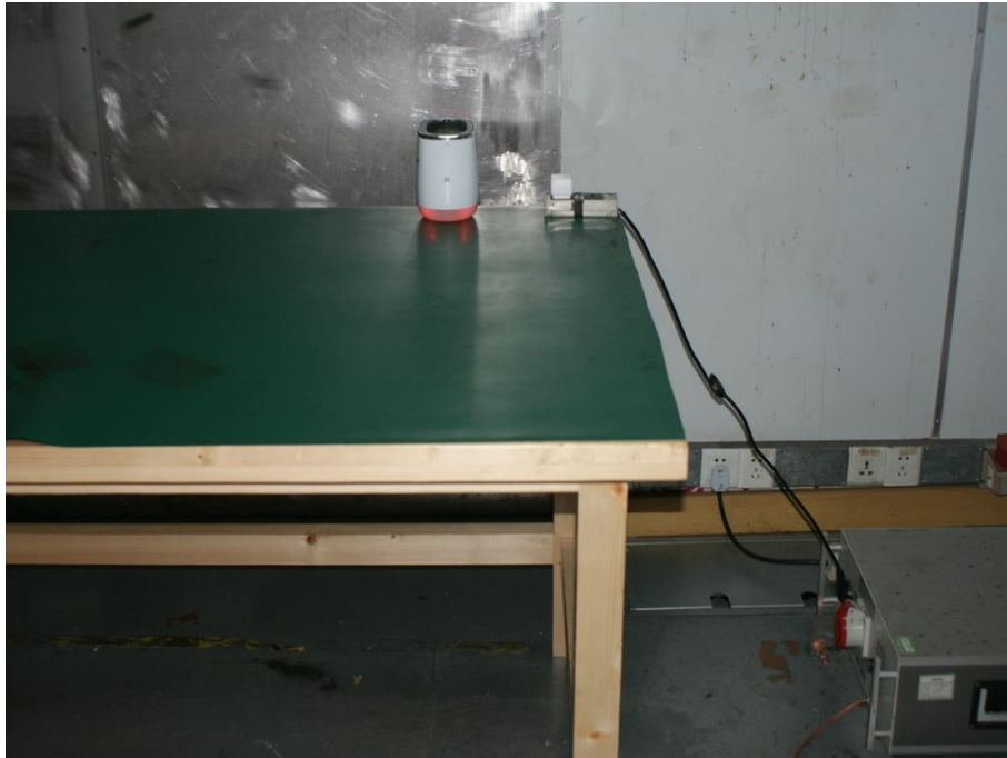
Photograph 7: Set-up for Radiated Emission (30MHz~1GHz)
