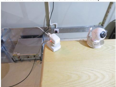
Radiated Emissions (30MHz-1GHz) Test Setup
