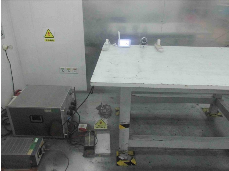
Photograph 4: Set-up for Conducted Emission on AC Mains
