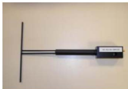
Figure 1 – Satimo COMOSAR Validation Dipole
