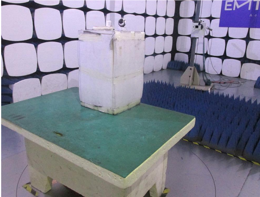
Photograph 3: Set-up for Radiated Spurious Emission, 18GHz - 26.5GHz
