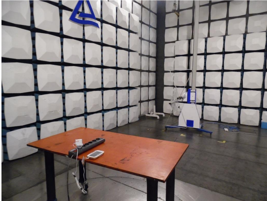
Photograph 1: Set-up for Radiated Spurious Emission, 30MHz - 1GHz
