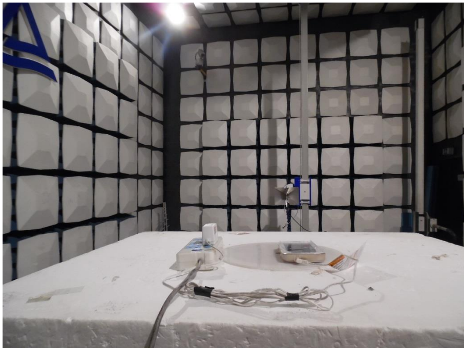
Photograph 2: Set-up for Radiated Spurious Emission, 1GHz - 18GHz
