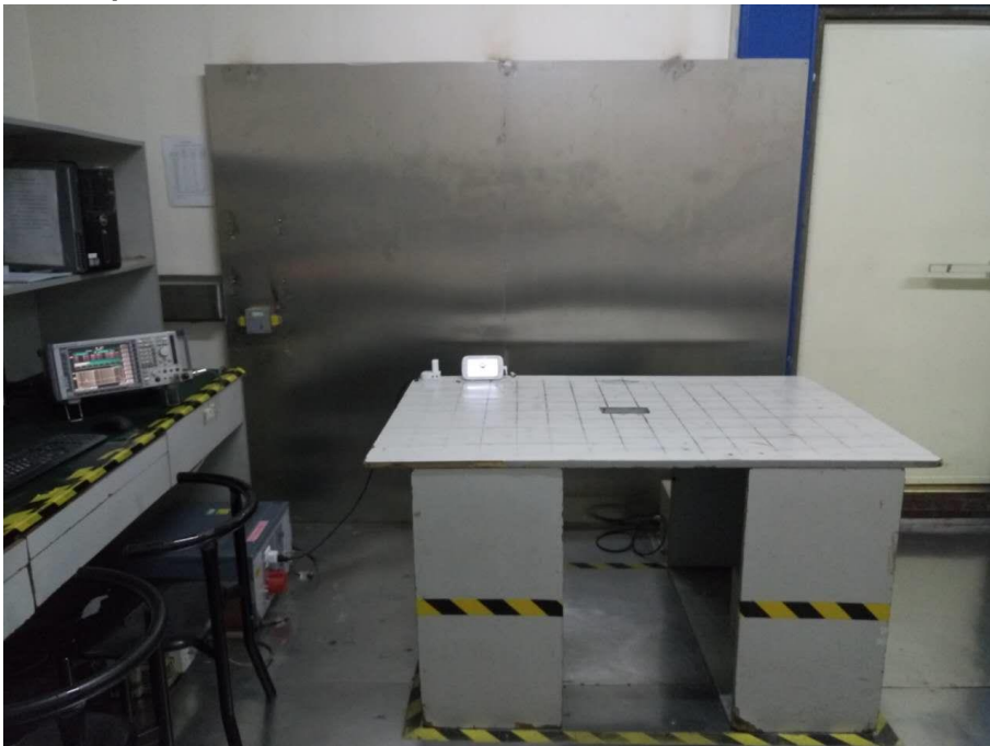
Photograph 4: Set-up for Conducted Emission on AC Mains
