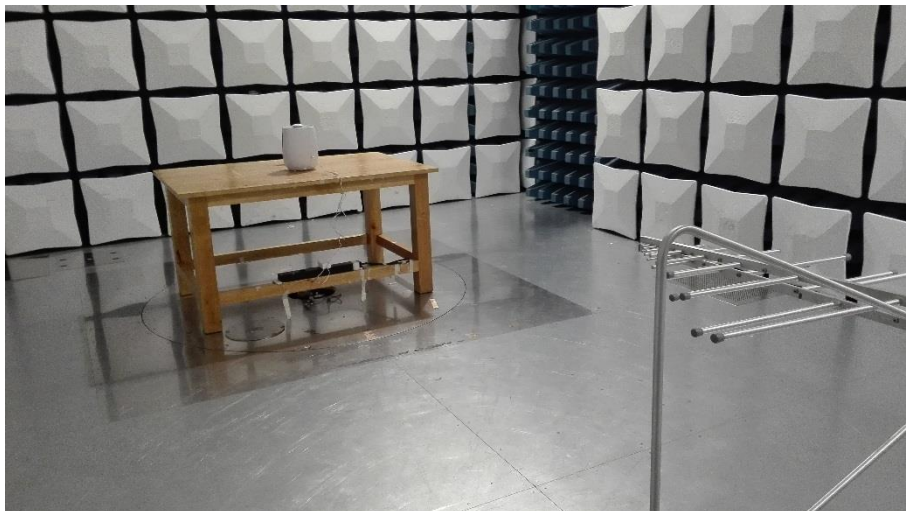
Photograph 2: Set-up for Radiated Spurious Emission, 30MHz ~ 1GHz
