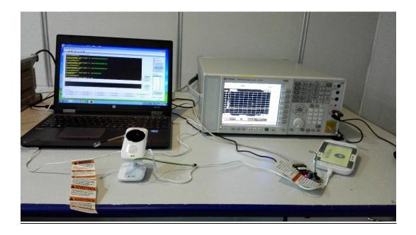
Photograph 2: Set-up for Radiated Spurious Emission, 30MHz~1GHz
