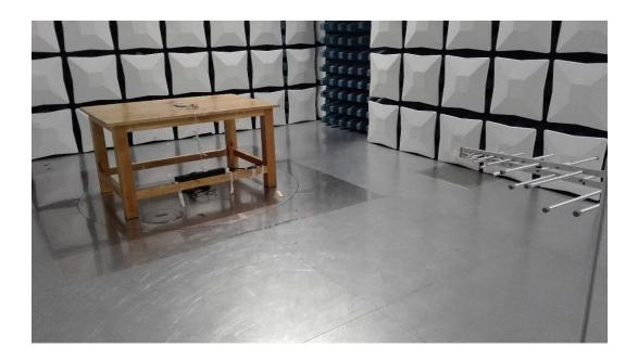
Photograph 6: Set-up for Radiated Emission, Above 1GHz
