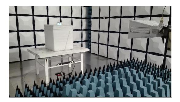
Photograph 4: Set-up for Conducted Emission on AC Mains
