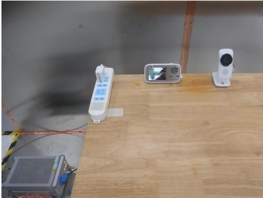
Photograph 3: Set-up for Conducted Emission on AC Mains
