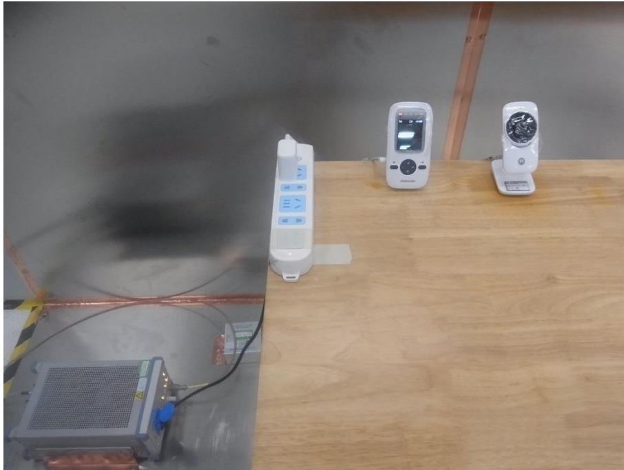
Photograph 3: Set-up for Conducted Emission on AC Mains
