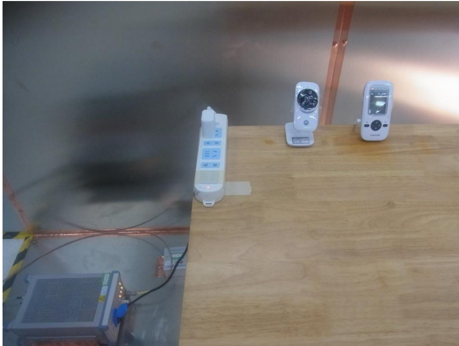
Photograph 3: Set-up for Conducted Emission on AC Mains
