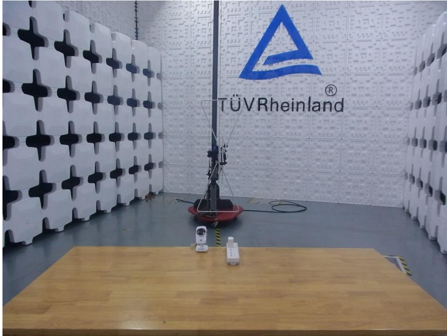
Photograph 4: Set-up for Radiated Emission, Below 1GHz
