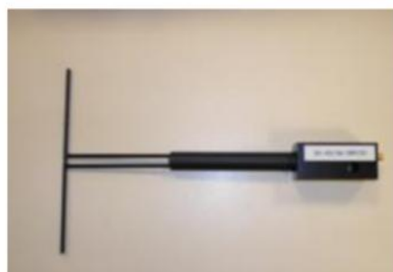
Figure 1 – Satimo COMOSAR Validation Dipole
