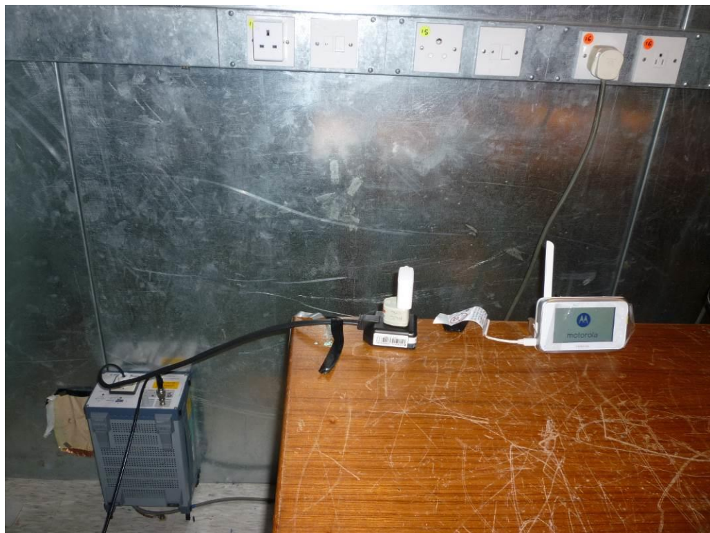
Set-up for AC power line Conducted Emission
