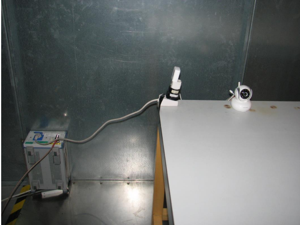
Set-up for AC power line Conducted Emission
