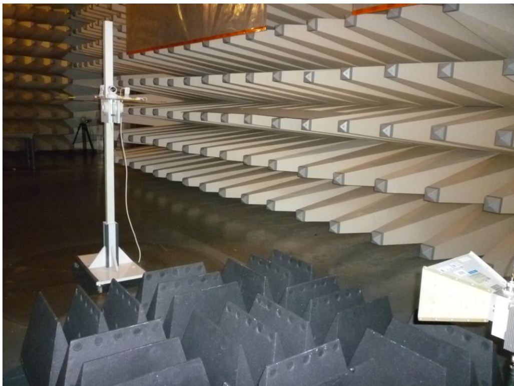
Set-up for Radiated Emission
