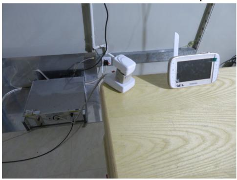
Radiated Emissions (30MHz-1GHz) Test Setup
