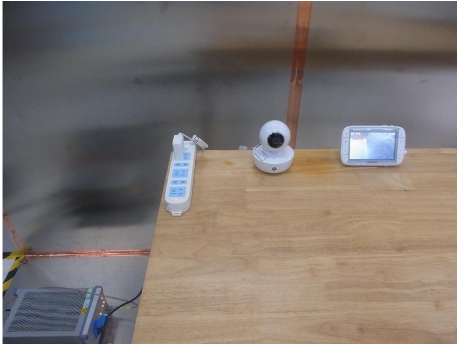
Photograph 3: Set-up for Conducted Emission on AC Mains
