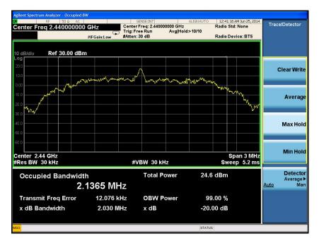
Result data graph shows 20 dB bandwidth, CF = 2440MHz, BW = 2.030MHz
