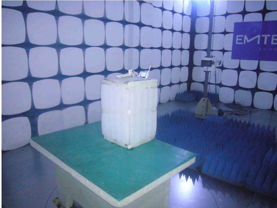
Photograph 3: Set-up for Radiated Spurious Emission, 1GHz ~ 18GHz
