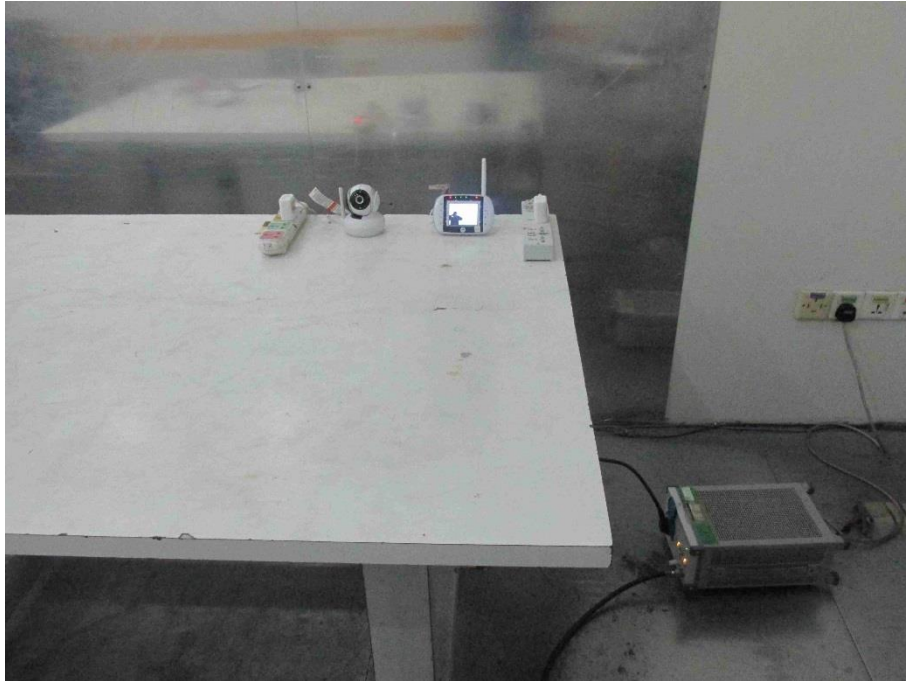
Photograph 5: Set-up for Conducted Emission on AC Mains
