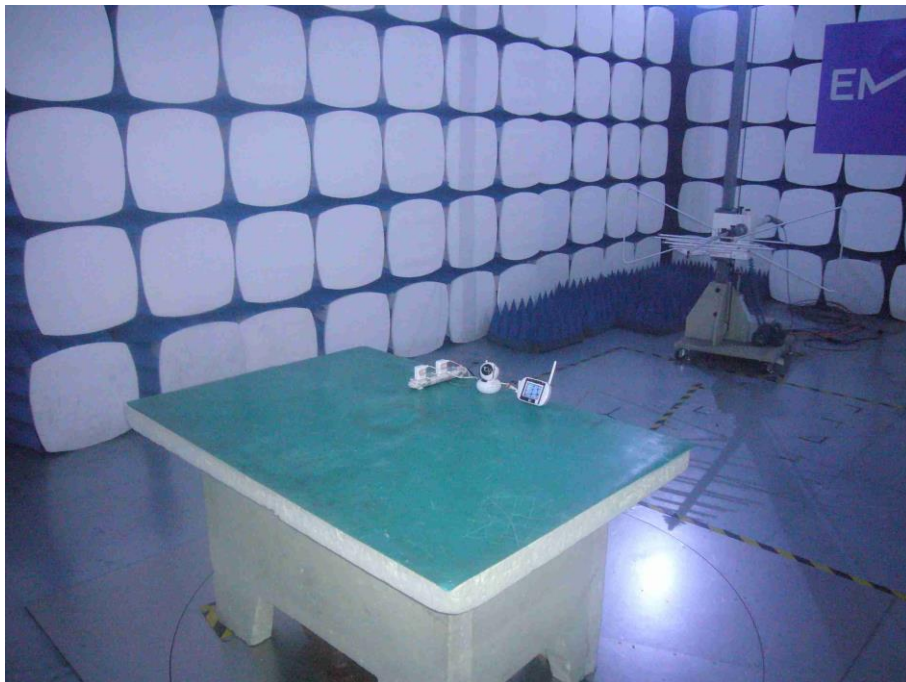
Photograph 6: Set-up for Radiated Emission, Below 1GHz
