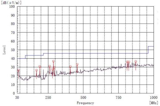
Radiated emission data graph (Horizontal polarization, 30MHz-1GHz)
