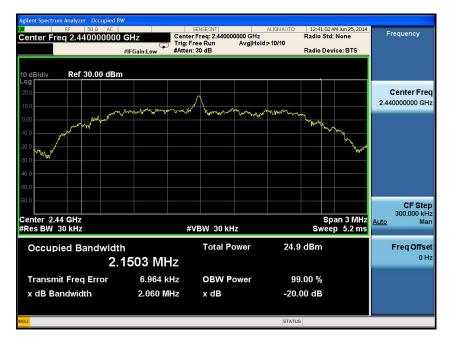
Result data graph shows 20 dB bandwidth, CF = 2440MHz, BW = 2.060MHz
