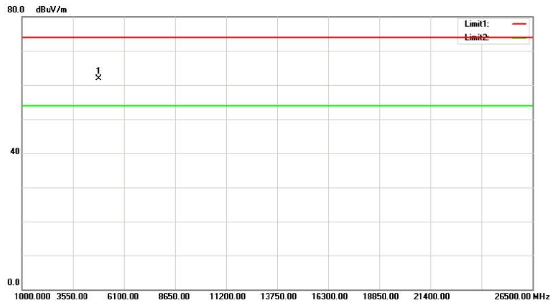
Figure 13 – Radiated emission data graph (Horizontal polarization, 1GHz-26GHz)
