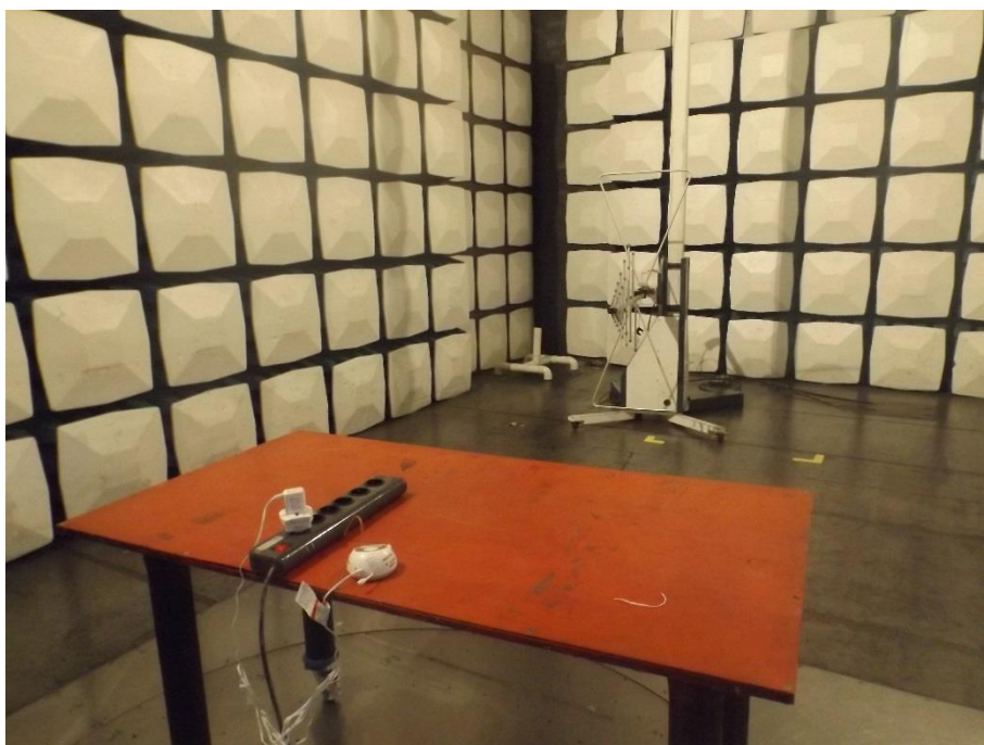
Photograph 2: Set-up for Radiated Spurious Emission, 30MHz - 1GHz
