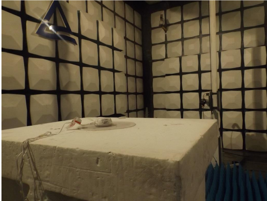
Photograph 3: Set-up for Radiated Spurious Emission, 1GHz - 18GHz
